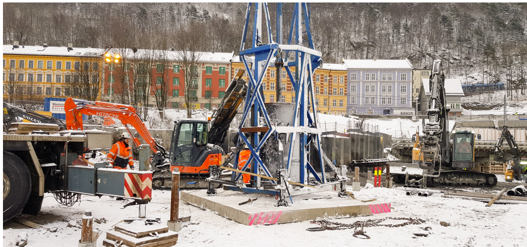
DLT with PP12 ; pile diameter=150mm; location: Oslo, NOR
